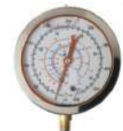
Pressure Gauge To keep a check on system pressure on low & high side
